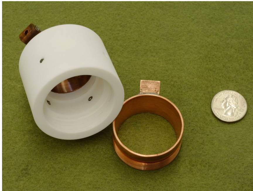
Figure E.8 The ends are not identical—the back side is the one with the spring-loaded bearings, as seen in this picture.
