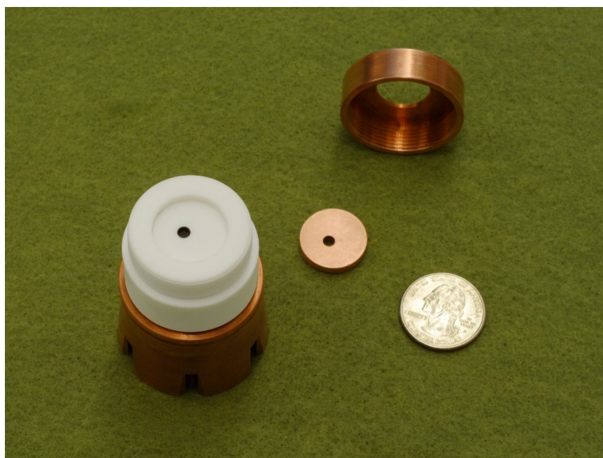
Figure E.2 The target and macor mask are placed onto the cathode base.
